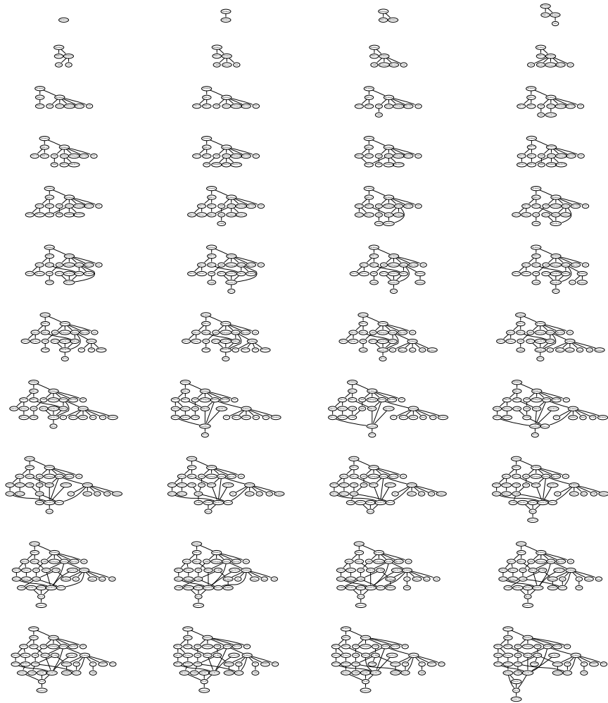
Fig. 2. Unix history graph. The first 48 frames drawn by serially inserting nodes with their incident arcs in breadth-first search order. Each frame is a readable diagram and the sequence appears somewhat stable.
